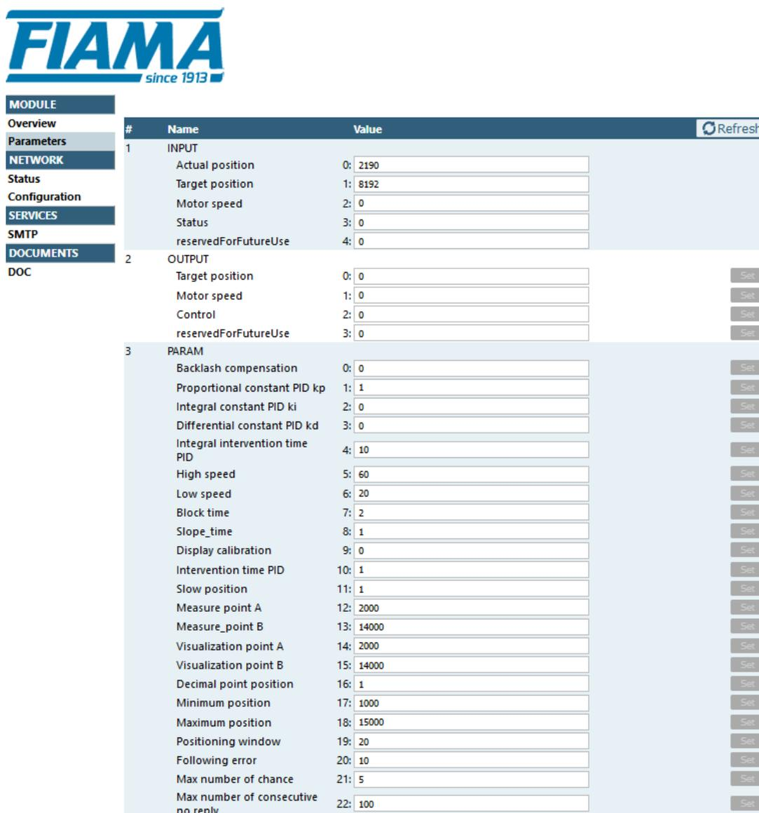
The screenshot shows the FIAMA web server interface. On the left is a navigation menu with categories: MODULE, Overview, Parameters, NETWORK, Status, Configuration, SERVICES, SMTP, DOCUMENTS, and DOC. The main area displays a table of parameters organized into three sections: INPUT, OUTPUT, and PARAM. Each parameter has a numerical ID, a name, a value field, and a 'Set' button. A 'Refresh' button is located in the top right of the table area.
