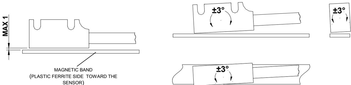
N.B. if the distance between the sensor and the magnetic band is over 1mm on the display appears **not APE**, and the measured value is wrong.
