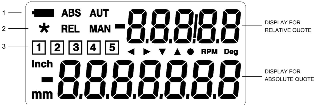
1. Indicator of flat battery: begins to blink when the level of loading goes under a certain value and when it keeps switched on its necessary to change the batteries within 1 month.
