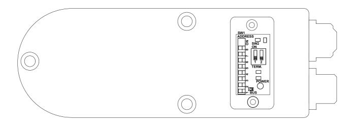
Set address and baud rate using dip-switch **SW1-SW3** as per following table:
