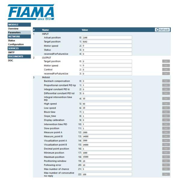
Using the web server it is possible to set the ServoDrive parameters using the PARAM. Section. Note: it is not possible to modify the input and output values, which can only be modified by a master device.
