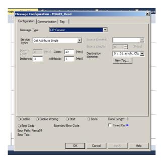
With this command (get), the entire block of parameter (50 byte) will be read and saved in the "destination element" struct.
