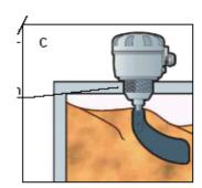
The level control has to be fixed on threaded hub 1"1/2 GAS, using a coupling or a lock nut (picture c).
